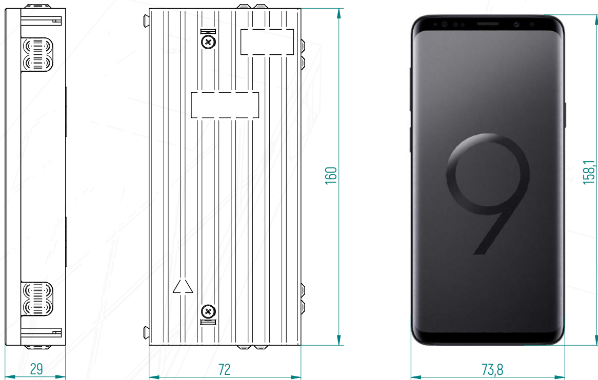
Picture 15. Comparison of box size to the popular smartphone on the market.
