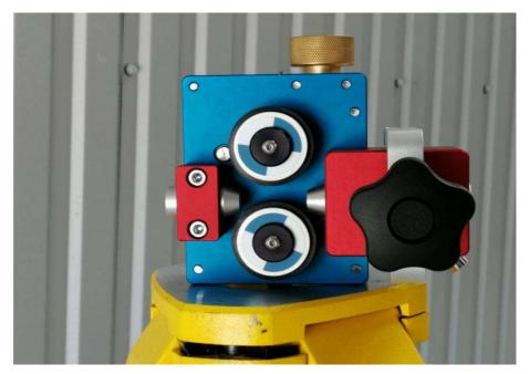
Lower the top drive roller onto the cable and press lightly. Depending on the clamping force and the friction factor between the cable and the rubber bands on the drive wheels, the pushing force is created.
