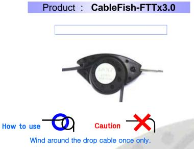
If you don't wind the drop cable, the tensile strength of cable will be reduced. ( Provided that you wind, the tensile strength will be 100Kg / If not, less than 40Kg )
