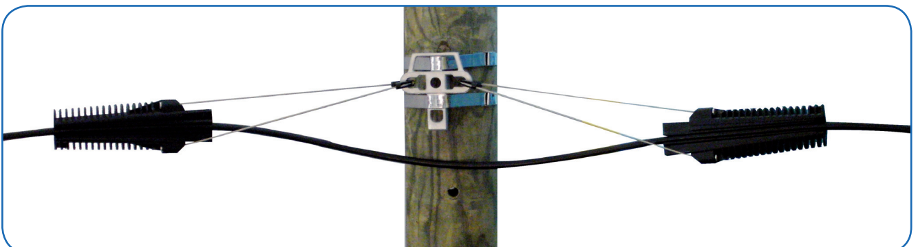
When the cable is brought to its installation load at the end pole, the wedges move further into the clamp body. When installing a double dead-end leave some extra length of cable between the two clamps
