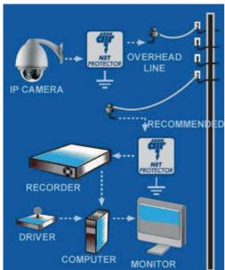
**AXON** *AIR* **Net***Protector* is designed to protect Ethernet 10/100/1000 Mb/s equipment connected with a twisted-pair overhead cable against impulse surges. The **AXON** *AIR* **Net***Protector* is the first stage of protection for overhead cable connections. It protects every wire in the four-pair cable and discharges the surge current to the ground. To work effectively the unit needs to be connected to the ground (never connect to the lightning conductor) or to a PE safety wire.
