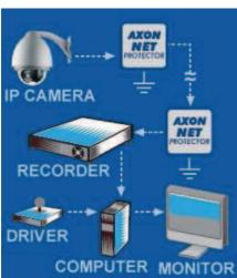
**AXON** Net*Protector* is designed for protection of Ethernet 10/100/1000 Mb/s network equipment against impulse surges. The used parts protect all four pairs of wires in the twisted-pair cables. Elimination of the surge between the lines is provided within each pair, and the occurring surge current is discharged to the ground through a PE wire. Such a solution guarantees effective surge protection.
