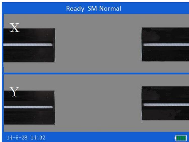
Close the lid of the Splicer and the EasySplicer PRO will move together the fibers and splice them together automatically. The whole process will be shown in the display (live video from both X/Y cameras) and take less than 10 sec. An automatic pull-test will be performed after the splicing. Finally, the splicer will show the estimated splice loss (in dB) or, if the process failed, "Bad splice" (if so, re-do the operation from "strip and cleave" above).
